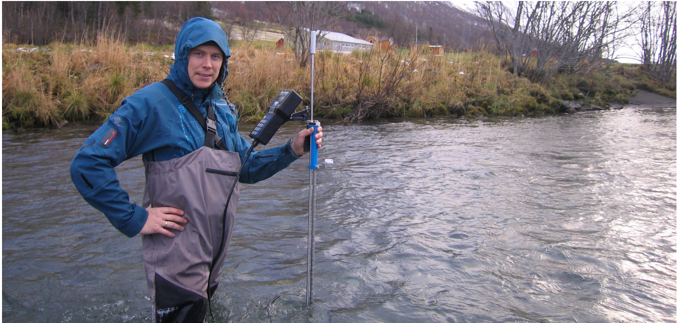
Research scientist Håkon Sundt from SINTEF carries out detailed measurements of the riverbed profile and water flow conditions. Together with laboratory experiments and numerical modeling studies, these field campaigns provide new knowledge on how hydropeaking affects fish and other living organisms in the rivers. Photo: Julian Sauterleute, SINTEF
