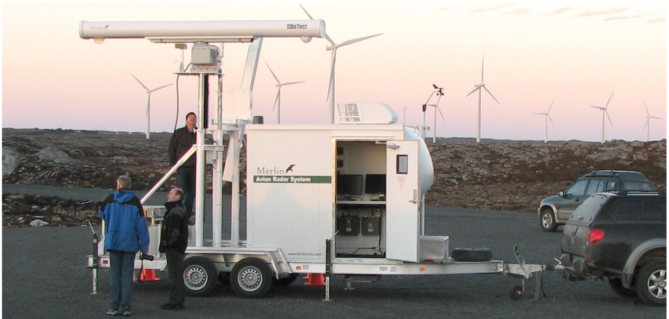
In March 2008 the BirdWind Project started to collect bird data on Smøla using the Merlin radar system at the picture. The experience acquired by the radar ornithologists is crucial also for the operation of a new car mounted 3D radar system. Photo: Kjetil Bevanger, NINA
