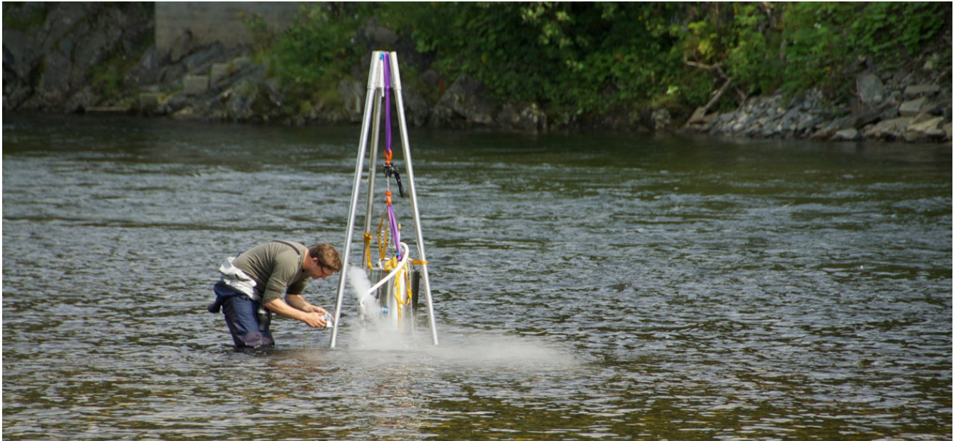
Ass. Prof. Nils R  ther works on sediment sampling by freeze coring in the River Surma. Photo: Nils R  ther, NTNU
