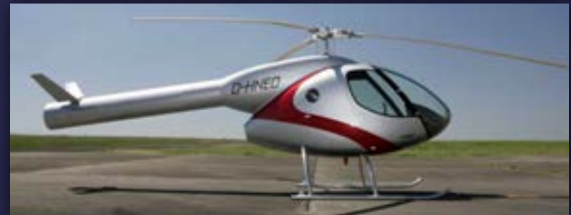
The NOTAR system used by NEO helicopter from YoungCopter
