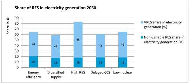
Figure 16: Share of RES in total electricity generation by the year 2050 in the five low-carbon scenarios, split in variable (here: wind and solar power, excl. small hydropower) and non-variable RES (hydropower, biomass, waste, geothermal). Source: [8].
