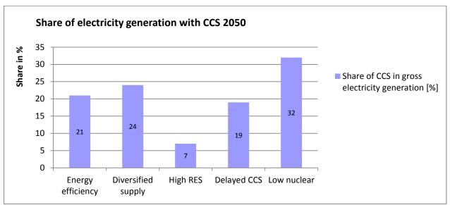
Figure 17: Share of electricity generation with CCS in gross electricity generation by the year 2050 in the five low-carbon scenarios. Source: [8].
