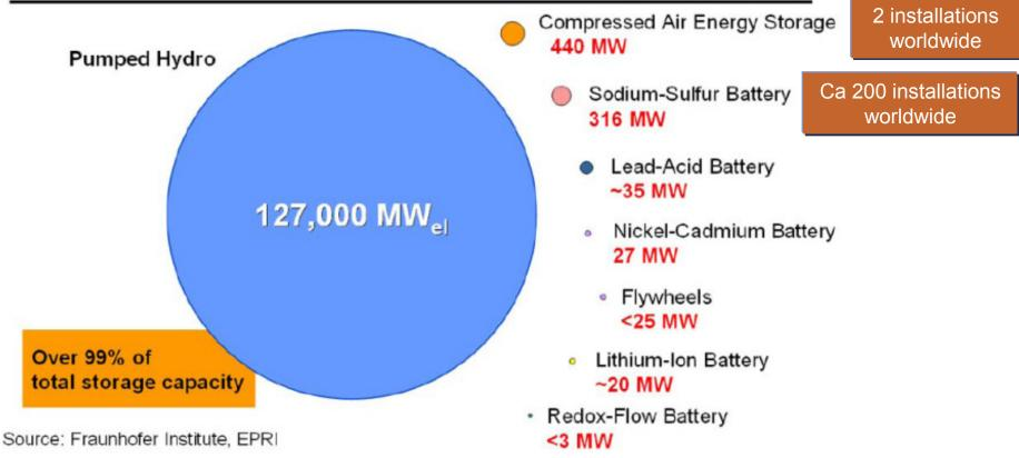
Worldwide installed rated power of storage facilities for **electrical energy**. Such power level can be sustained for up to several hours or shorter
