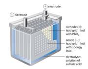
cell reaction: Pb(s) + PbO<sub>2</sub>(s) + 2HSO<sub>4</sub>  $^{-}(aq) + 2H^{+}(aq) \rightarrow$ 2PbSO<sub>4</sub>(s) + 2H<sub>2</sub>O(I)
