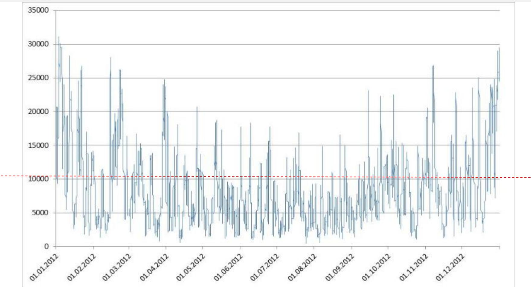
Observed Wind energy production in a system with **45600 MW** installed capacity (Stadium 2012)
