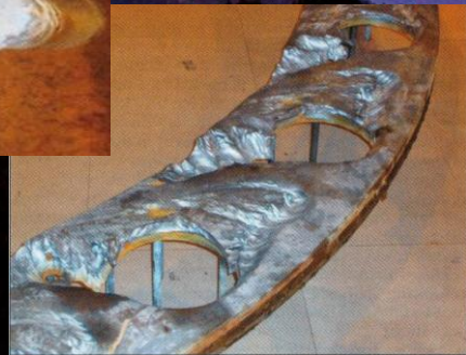
Sediment erosion in guide vanes and facing plates
