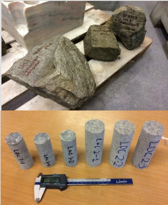
Cores, extracted from the samples collected from field and ready for UCS Test
