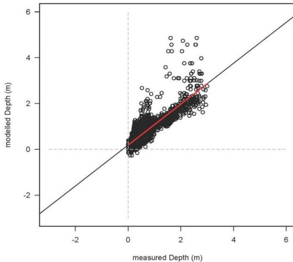
Method by Lyzenga (1981) and Flener (2013): Removes all information from the image that is not "depth" (e.g. substrate colour, turbidity); requires some directly measured depth values for calibration.
