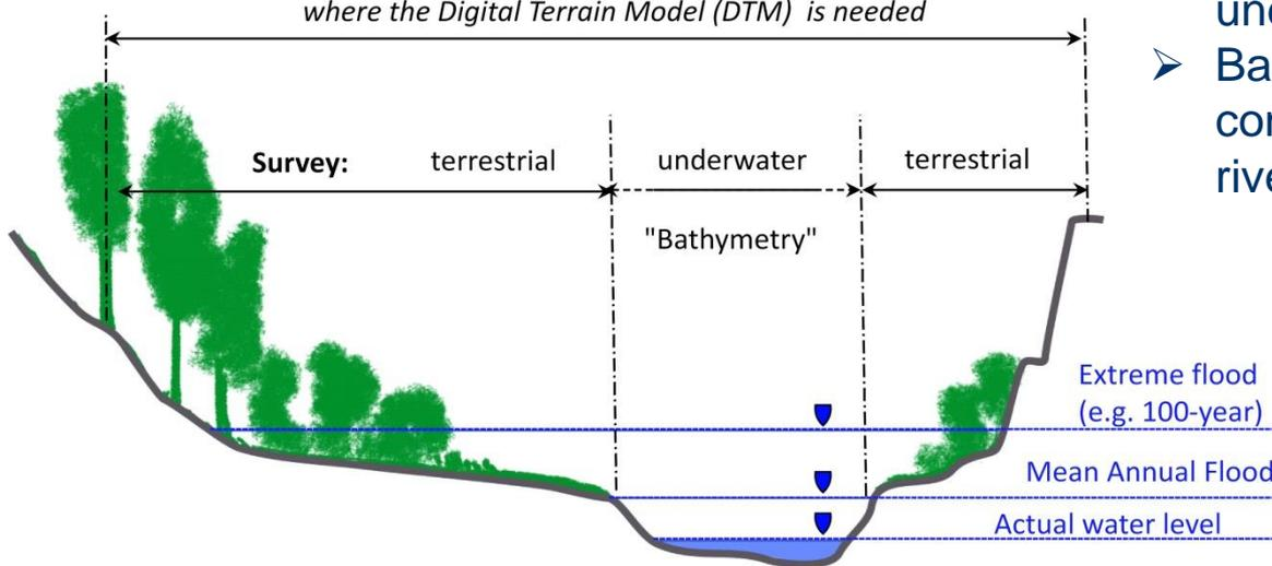
**Bathymetry = the underwater equivalent to topography in oceans, lakes and rivers**
