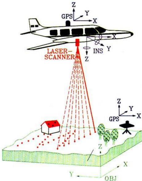
*Laser measures aircraft-ground distance with high accuracy; Reflections from vegetation etc. have to be filtered out*
