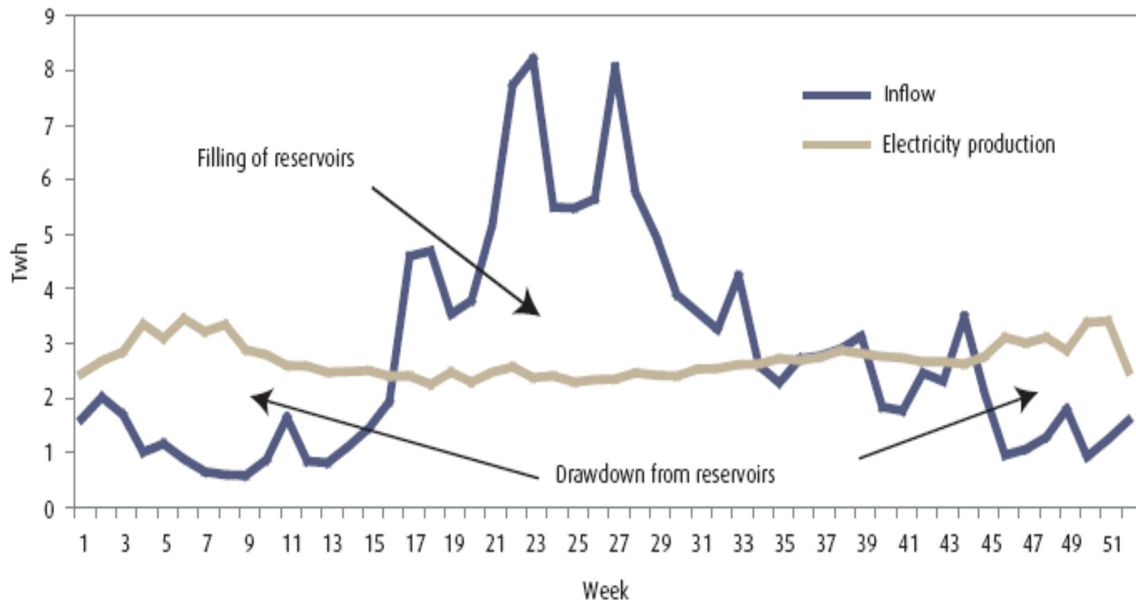
Figure 2.2 Variations in water inflow and electricity output in 2007.
