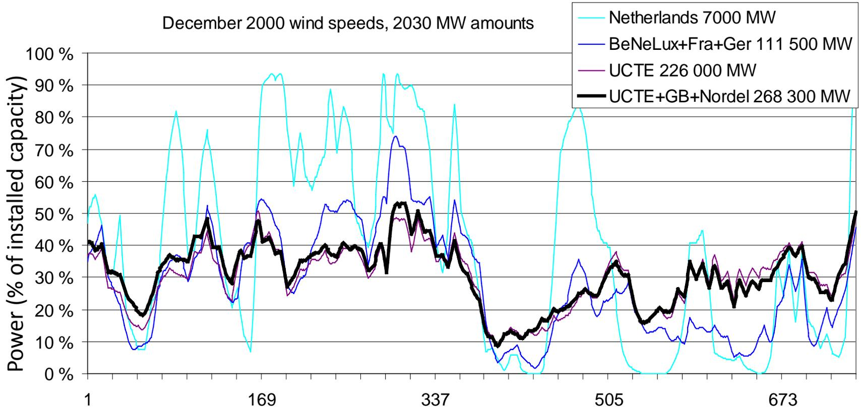
*Pan-European balancing can reduce storage needs of wind+PV by a factor of 11 compared with regional storage*
