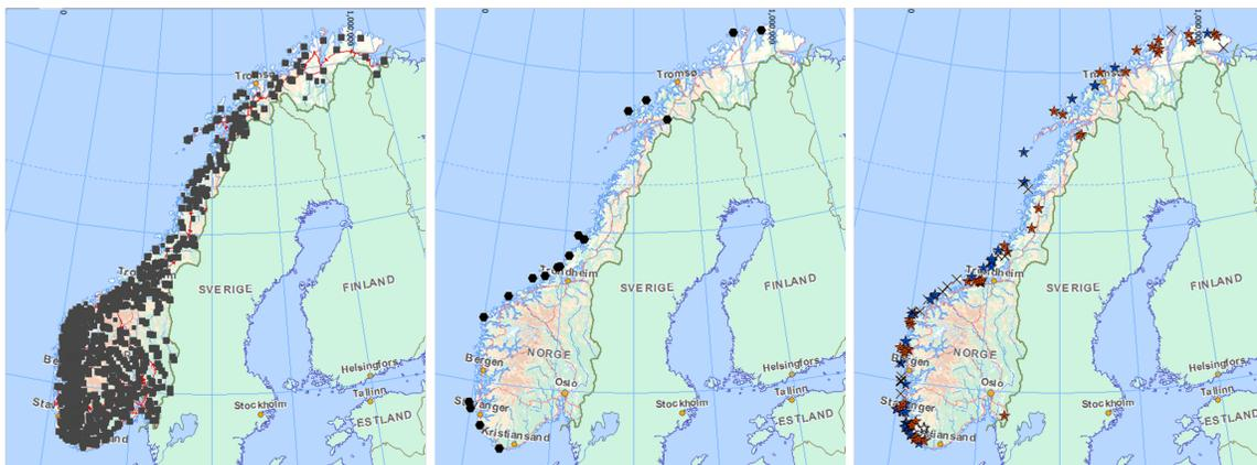
Figure 1-1: Left: Developed hydropower stations. Middle: Developed wind power sites. Right: Proposed wind power sites. Image source: NVE Atlas [www.altas.nve.no](http://www.altas.nve.no)
