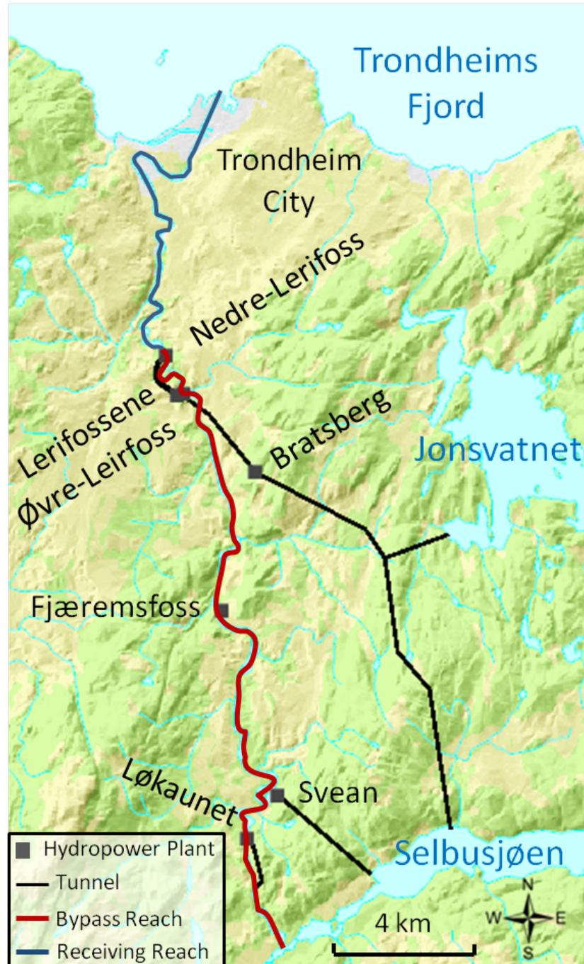
Figure 2-2: Map of the River Nidelva, flowing from Selbusjøen reservoir to Trondheimsfjord. The bypass (red) and tunneled (black) pathways feed into the receiving reach (blue). Note that the tunnel from Jonsvatnet to Bratsberg is not in use.
