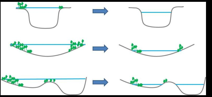
Shape of reservoir s determines the biological impact when the waterlevel is reduced. The plants illustrates the littoral zone.
