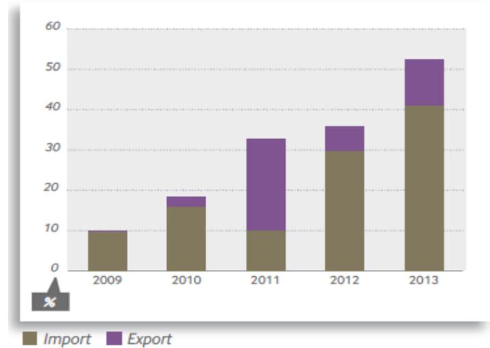
**Frequency of saturation of FR→DE interconnexion (in %) – 2013 – source : RTE**
