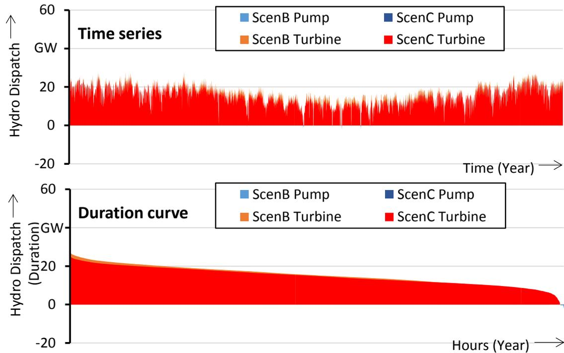
Figure A.3: Dispatch of hydropower in Norway without additional transfer capacity
