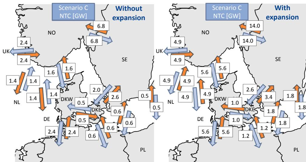
**Figure 4.4: Comparison of transfer capacities with and without expansion of hydropower and transfer capacities in scenario C**
