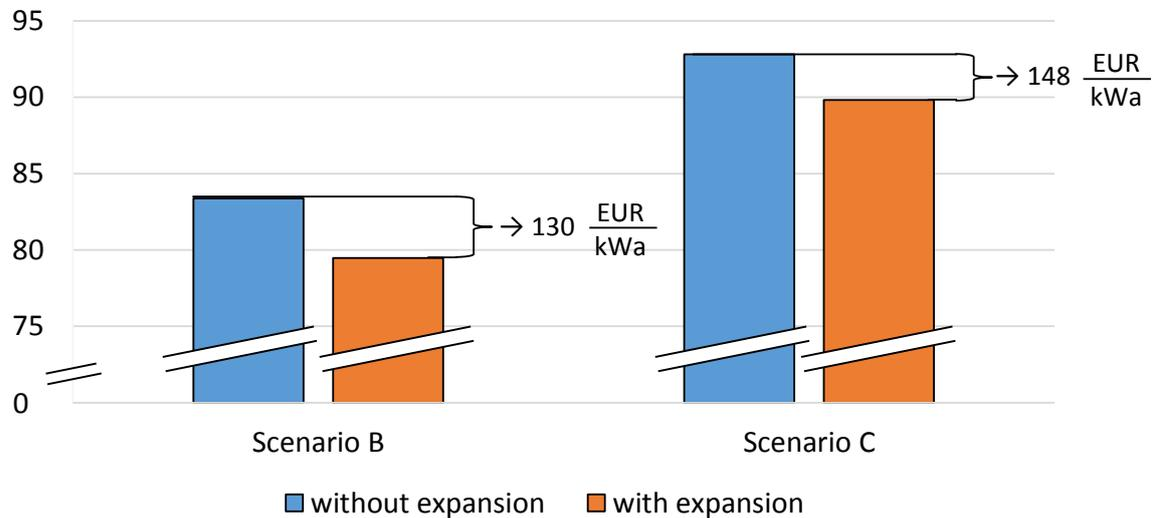
**Figure 5.3: Impact on variable system cost by additional hydropower capacity**
