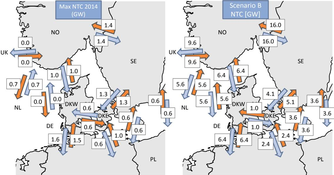
Figure A.1: Transfer capacities from and to Scandinavia in comparison to 2014 NTC values
