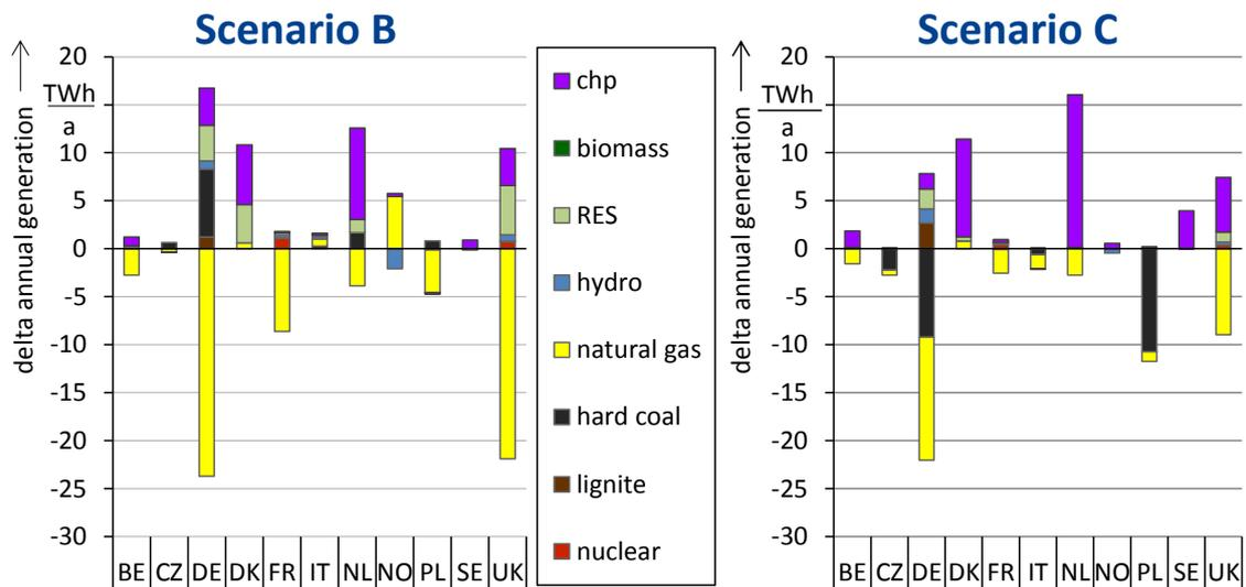
**Figure 5.1: Difference in power generation with additional hydropower capacity in Norway**
