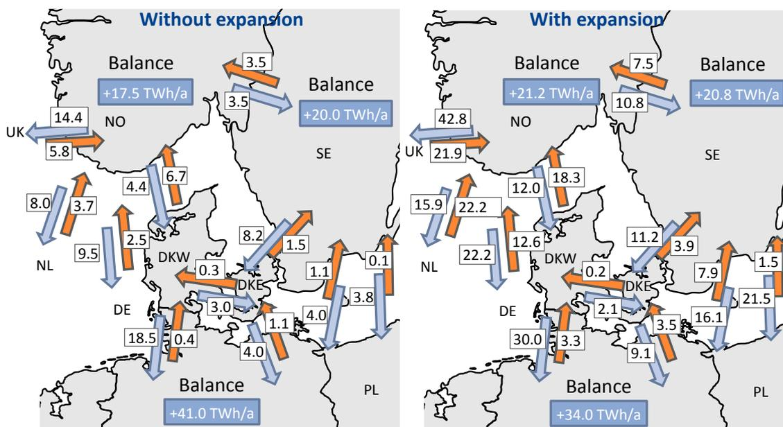
**Figure 5.2: Power exchanges with and without hydropower expansion in Norway in [TWh/a] (scenario B)**
