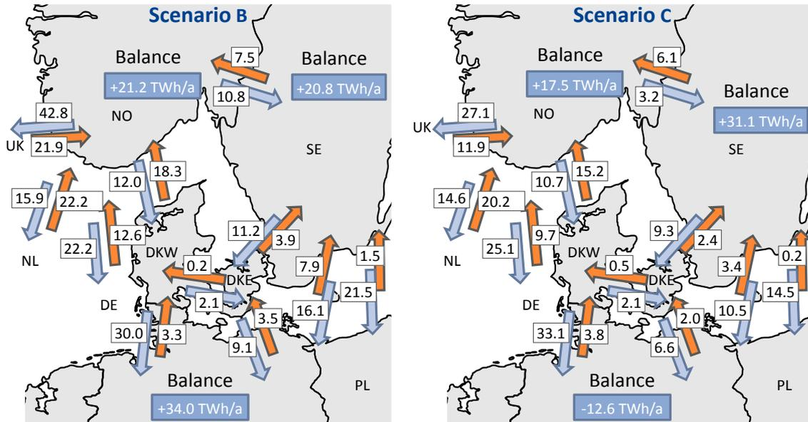
**Figure 5.8: Power exchanges from and to Scandinavia in [TWh/a]**
