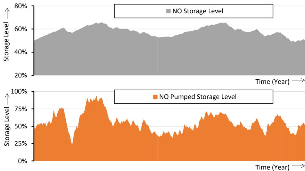
**Figure 5.12: Dispatch of Storages and Pumped Storages in Norway in Scenario B**
