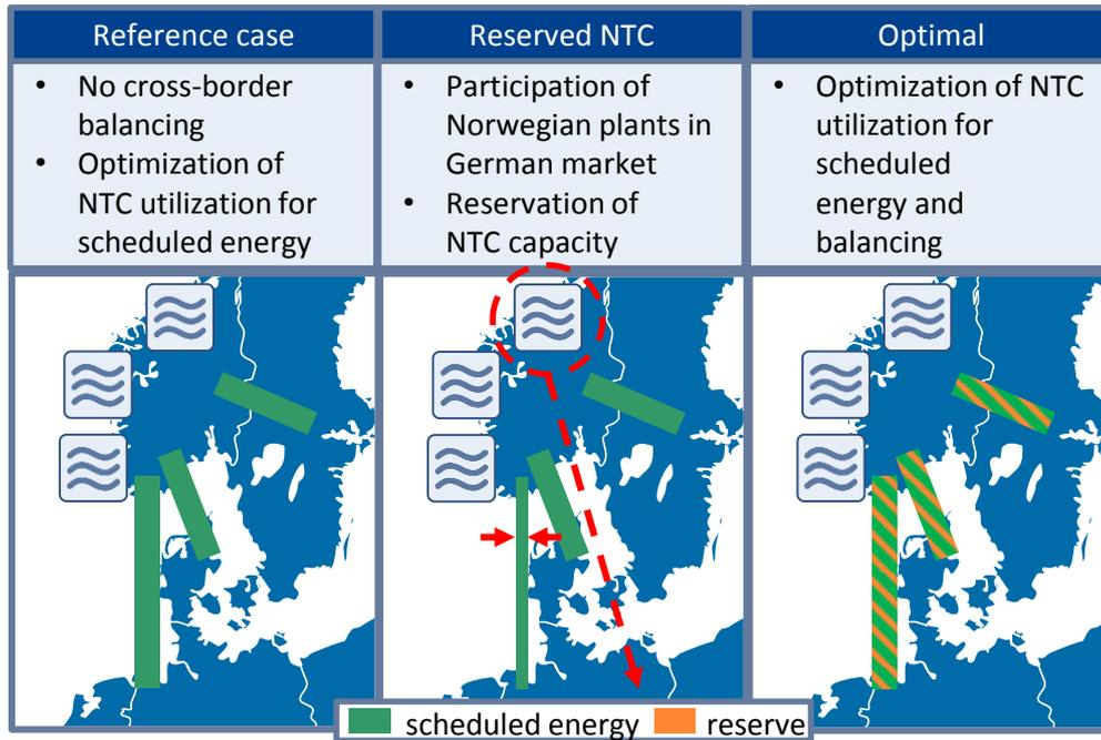
**Figure 2.2: Cases for the utilization of cross-border capacity**
