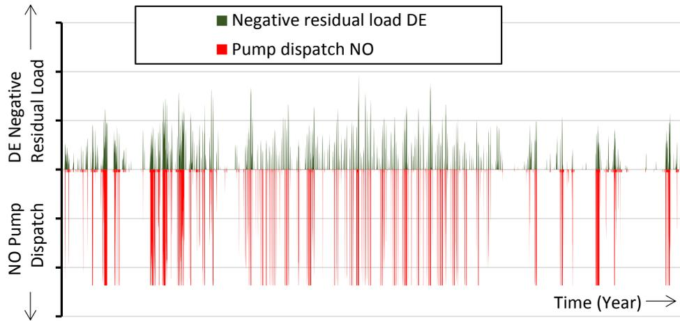
**Figure 5.11: Correlation of Residual Load in Germany and Norwegian Pump Dispatch (scenario B)**
