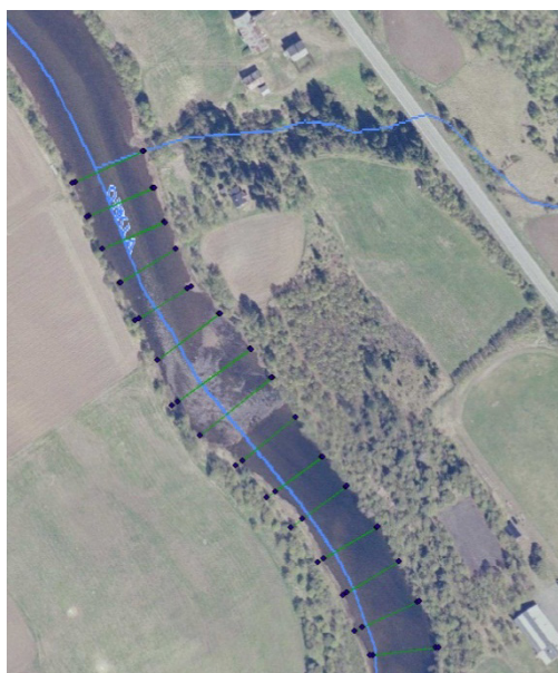
Figure 3-15. Extracted transects (left) and histogram of wetted widths (right) for Orkla, station 121.25, discharge 5.07 \text{ m}^3/\text{s} , based on the aerial image from 30.05.2004. The site is influenced by small weirs.
